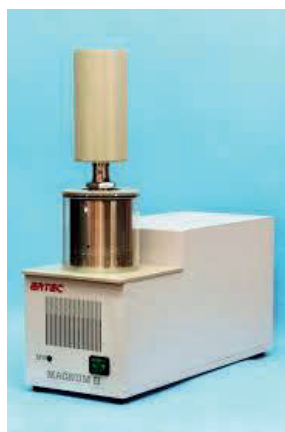
Figure 1. Microwave-driven hydrothermal reactor Magnum Ertec II.
